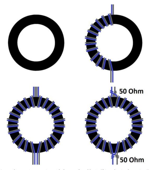
We start by securing two wires with the use of a cable tie. This makes it a lot easier. Keep to the bottom about  $5\ \mathrm{cm}$  wire length, this is enough length.
