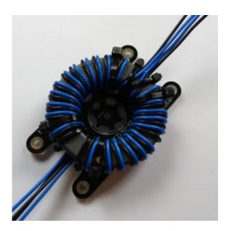
Connect the primary side of the ring core (bottom, where the blue wires are next to each other) to the coax connector. The two blue wires at the center core of the coax connector and the black wires on the chassis part with a cable lug. Remove the plastic parts from the cable lug so that a solid solder connection can be made.
