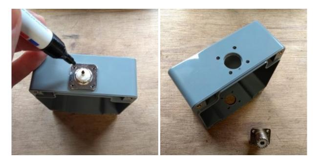
After all the holes are drilled, both connectors can be mounted as shown in the picture below. Don't forget to mount the M3 cable eyelet to one of the four screws.
