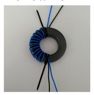
Then wrap 12 windings on the second half. Note that the wires are wrapped exactly as in the example. Do not change colors or wrapping directions. At the bottom of the toroid the two blue wires are next to each other and the black wires on the outside. At the top of the ring core, this is exactly the other way around, there are the black wires next to each other in the middle and the blue wires on the outside. If this is not correct, start again because then something went wrong.
