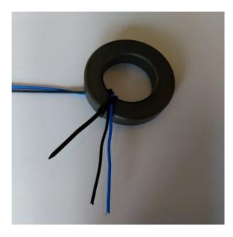
Then wrap the first 12 windings on half of the toroid as shown in the picture below. Make sure the windings are tightly placed together.
