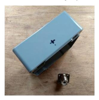
After the 16 mm holes have been drilled, I put the chassis part in the hole to determine the position of the fasteners holes. I picked a chassis part where I fix the part with 4 screws, but 2 screws could also work. These holes can be drilled with a 3,5 mm drill.
