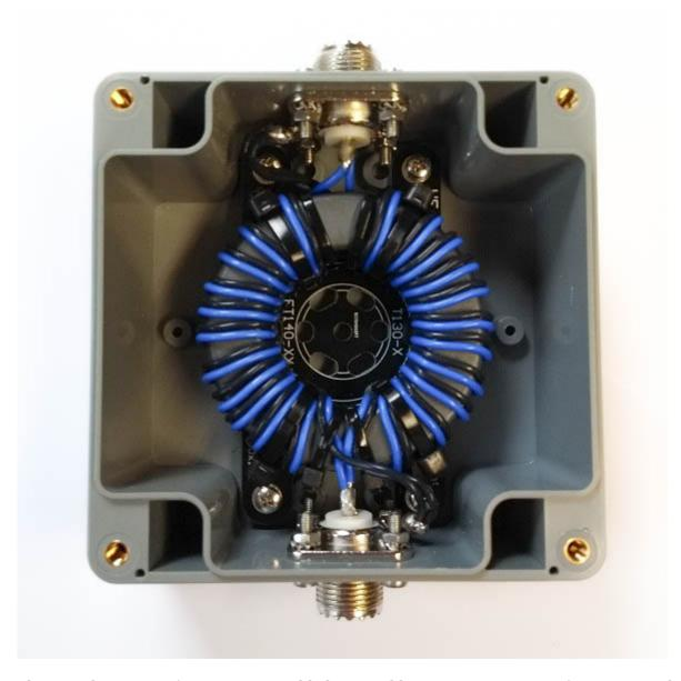
The impedance transformer can possibly be tested by putting a resistor of approximately 50 Ohm (e.g. 47 ohm) over the output connector. Then the SWR meter should show a standing wave ratio of 1:1. Of course, a "dummy load" can also be used for testing purposes.
