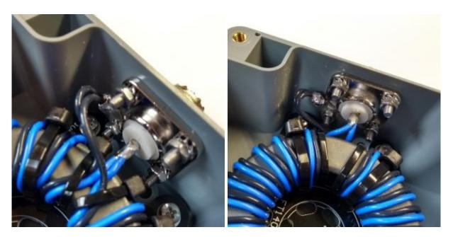
Now connect the other side of the toroid core to the coax connector. The two blue wires at the center core of the coax connector and the black wires on the chassis part with a cable lug.
