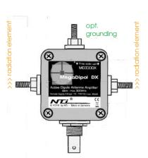
The radiators are fixed to the two M5-screw connectors on the side of the unit using tooth lock washers and wing nuts. It is important to install the antenna case with the BNC-connector pointing downwards because there are two small holes to allow condensation to exit.
