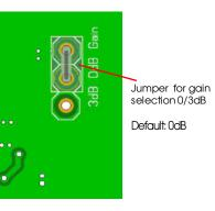
Within the antenna case, there is a jumper for selection of optimum gain.
